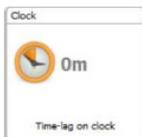
This icon indicates the time drift between the radar speed sign and the computer. A simple click will allow you to synchronise the times of the radar speed sign and the computer.
