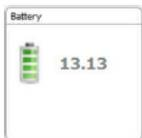
Battery level indication. If the battery level is low, the icon changes colour. A fully charged battery is between 12.8 V and 13.1 V
